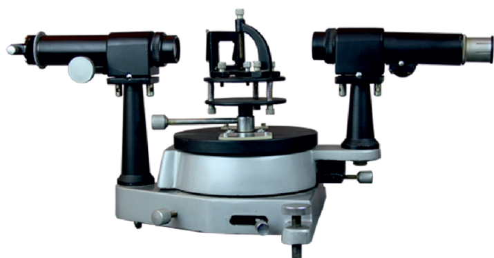
a) SMB-1708/1 - Student spectrometer routine quality 6"
