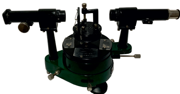
b) SMB-1708/2 - Brass movements superior spectrometer 6"
